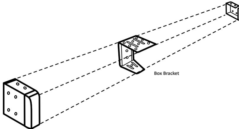
If more than one center wide support bracket is provided, they should be spaced evenly between the two mounting brackets.
